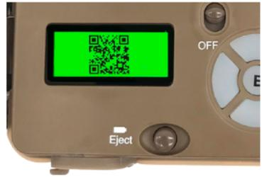
Press the MODE button to return to the main menu. Use the UP arrow button and scroll to the LTE Info menu option. Press the ENTER button to display the camera’s ICCID. This is the ID for the SIM card for the carrier you selected.
