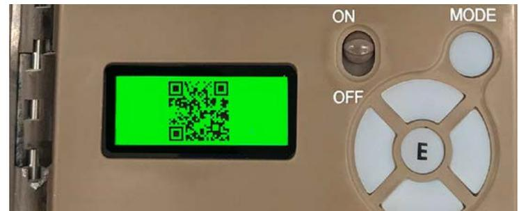
A QR code will appear on the camera display screen. Open your Strike Force Wireless app on your mobile device. Simply choose the "ADD CAMERA" option in the App located as a '+' symbol in the upper right corner of the 'Cameras' screen. A QR code scanner will appear on your screen. Scan the QR code displayed on the camera screen with your mobile device.
