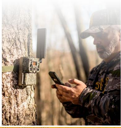
Your camera will make connection with a cell tower and transmit the images to your Strike Force Wireless account. You can view the pictures on your laptop or mobile app. Your camera screen will display the cellular signal strength. If your camera registers the cell tower strength low, you may need to relocate the camera to an area with a stronger signal.
